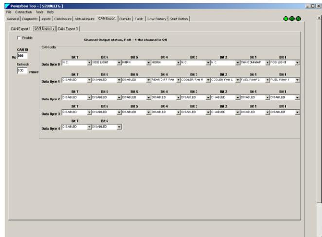
If for example channels assigned to bit 2 and 6 are ON and all other channels are off, the byte value is 68.
