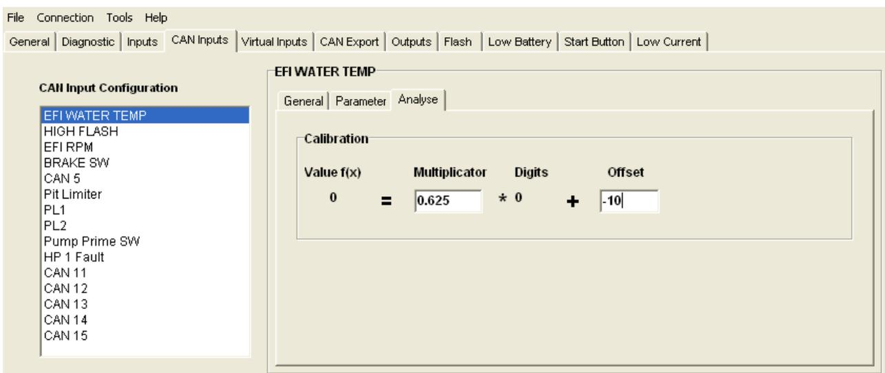
The multiplier is the increase in engineering value per bit and the offset adjusts the channel's value at zero bit.
